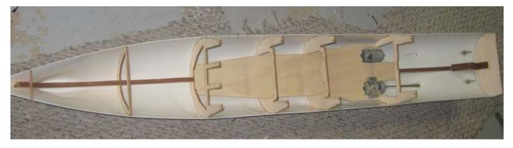
I then drilled the holes for the rudder stuffing tubes and the propeller shafts. I installed the motors and discovered that the motor shaft does not line up with the propeller shaft. I ordered two Robbe gear motors which have a offset output
