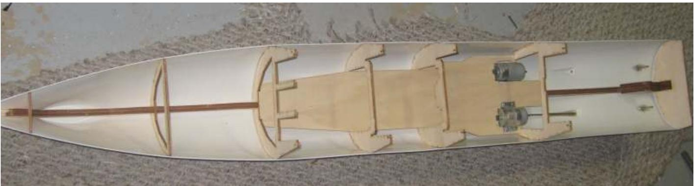
I then drilled the holes for the rudder stuffing tubes and the propeller shafts. I installed the motors and discovered that the motor shaft does not line up with the propeller shaft. I ordered two Robbe gear motors which have a offset output
