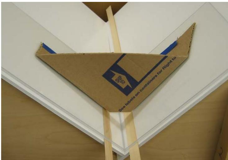
Figure 13. Cardboard buttress to support glued sides.
