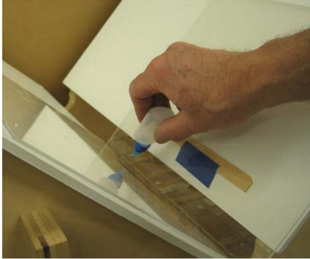
Figure 11. Applying glue with a hypodermic-tipped bottle.
