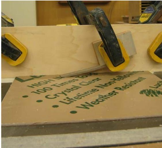
Figure 5. Hold-down to keep acrylic flat across the blade.
