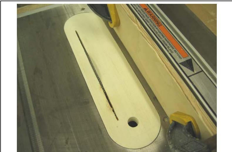
Figure 4. Zero-tolerance insert for table saw.
