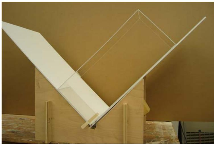
Figure 14. Case in jig ready for final gluing.
