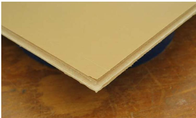
Figure 6. Finished rabbets with flat kerf and even depth.
