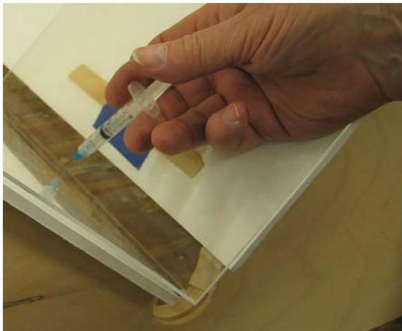
Figure 12. Applying glue with a hypodermic-tipped syringe.
