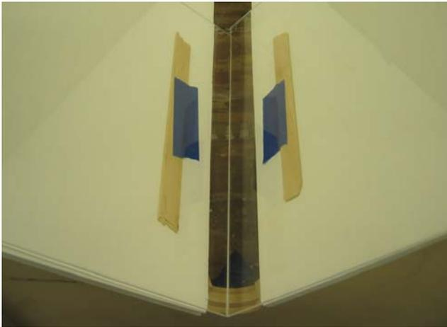
Figure 9. Thin sticks used to elevate the acrylic away from the jig.
