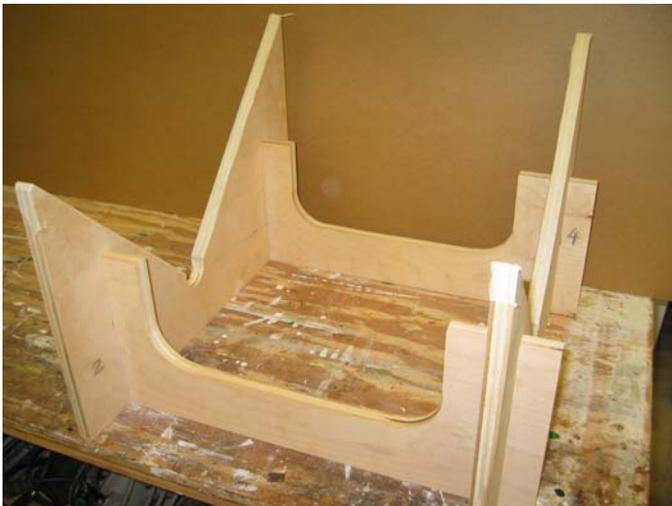
Figure 9b. Side view of assembly jig.
