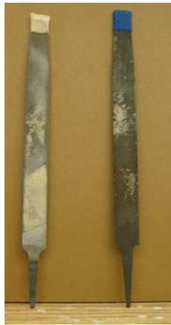
Figure 15. Bastard-cut and mill-cut files, with taped ends to avoid scratching and gouging of the acrylic.
